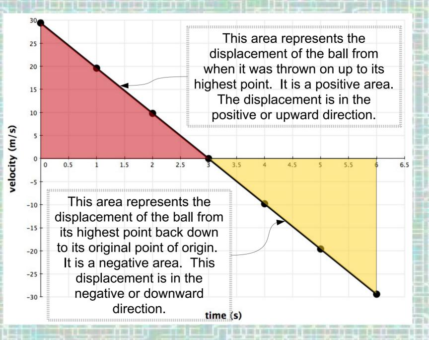
Here's the upward displacement which occurs during the first 3 seconds.  $A = \frac{1}{2} b \times h$  $A = \frac{1}{2} (3.0 \text{ s})(29.4 \text{ m/s})$ A = +44.1 meters
